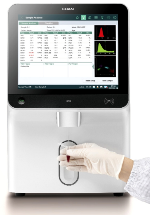
16µL microliter of sample aspiration
